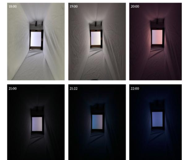
Prototype phase 2. On six occasions between 18:00-22:00 photos were taken of the transitioning light through the glass. The color was taken from the visualisation. An Atom Matrix, two RGBW led were used to conduct the test.
